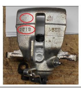
Cores which are not of OE origin or are not supplied by FTE with approved marking will be rejected and scrapped on site.
