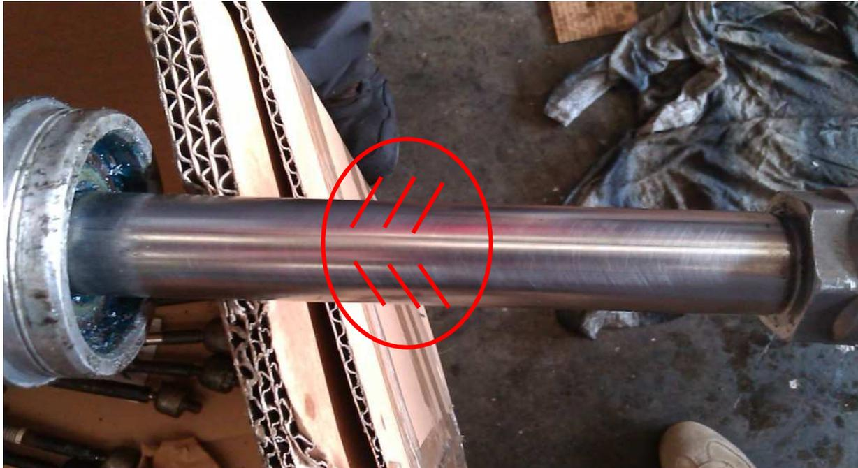
**The red circle shows that the rack has been filed / eroded : in this case, the diameter is smaller than the original, and in this case we will not be able to use the original components / rubber seals because it has been modified.**
